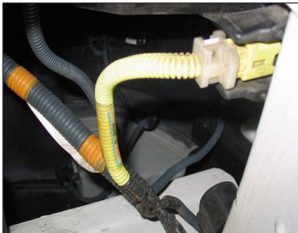
Example SRS Wiring (yellow)
